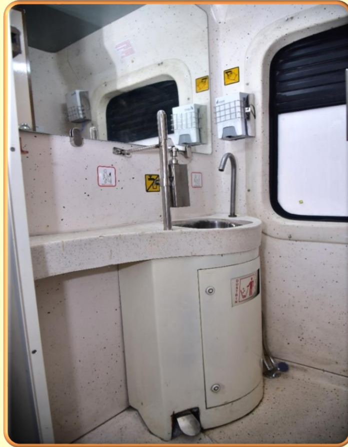
Foot operated water tap & soap dispenser
